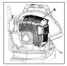
Removal of cooling passage blockages or cleaning of cooling fins is considered normal maintenance. Any failure attributed to lack of maintenance is not warranted.
