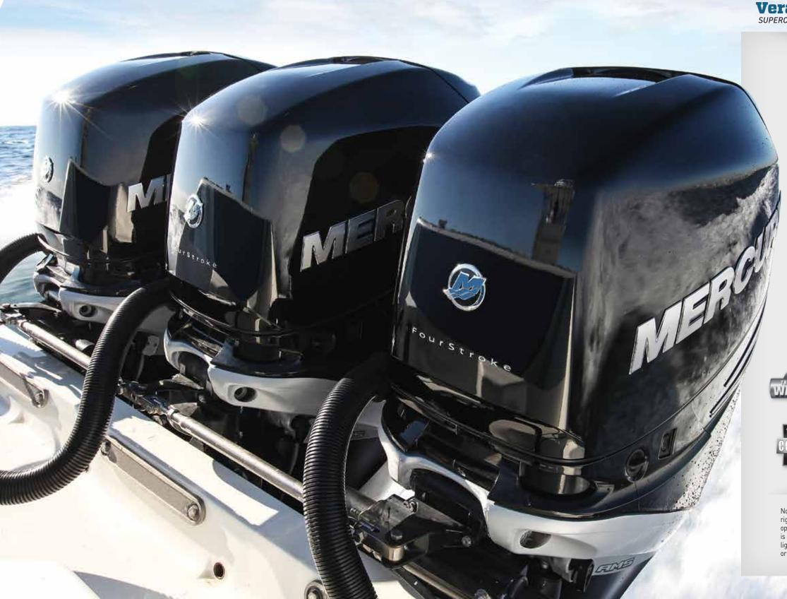
350 Horsepower Full Throttle RPM 5800-6400 I-6, 24-valve, DOHC Engine Type Displacement 158.5 cu in (2.6L) Supercharged w/charge air cooling Induction System Starting SmartStart electric Gear Ratio 5.44 in (1.75:1) HD Alternator Output 70 amp (882 watt) SmartCraft programmable trim and tilt Trim System Dry Weight\* 668lbs (303kg) Electro-hydraulic power steering Steering 20 in (508mm) CR 25 in (635mm) CR Shaft Length 30 in (762mm) CR
