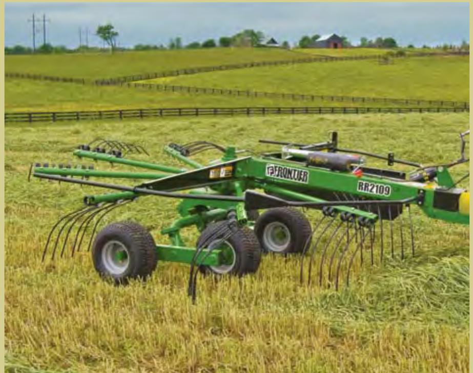
Ideal for small hay producers with minimum 30 PTO HP tractors, the RR2109 Rotary Rake has a 9-foot raking width.
