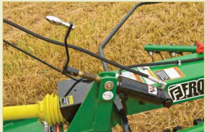
Make quick and easy adjustments with the rake-leveling cylinder. Designed for drawbar height variations, the rake-leveling cylinder features a manual tilt adjustment that allows you to fine-tune pitch.
