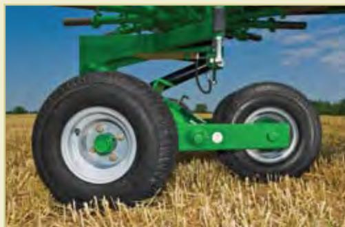
Tandem axle walking beam helps the rake stay level over uneven terrain, preventing hay loss when raking. And four large flotation tires reduce soil compaction and provide a smooth ride over rough ground.
