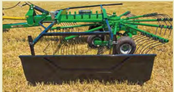
Heavy-duty vinyl curtain is easily adjustable to set your desired windrow width. Or simply remove the curtain to combine multiple windrows.
