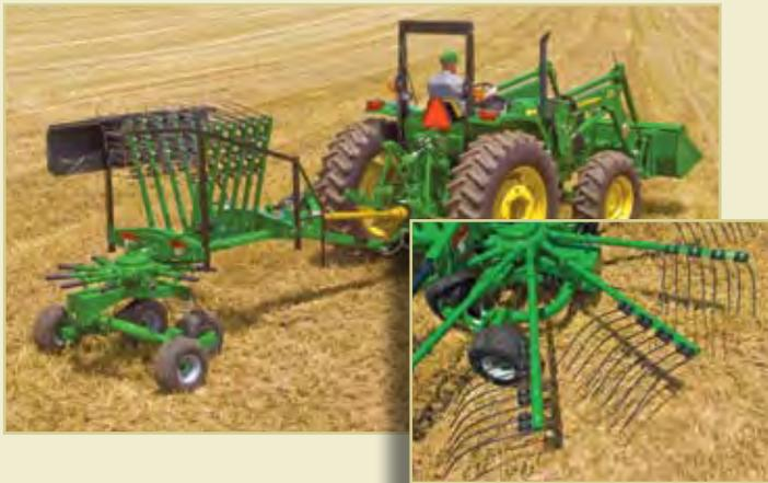
The RR2211 is set with 11 removable tine arms. The tine arms can be manually detached and positioned upright for easy transport and convenient storage.
