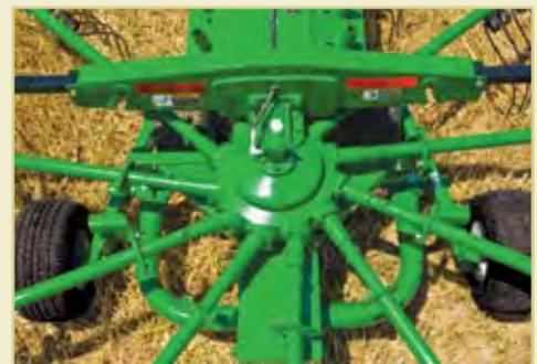
Both models of Frontier Rotary Rakes are equipped with a fully enclosed gearbox to keep dirt, debris, or hay from getting inside. This feature allows for improved reliability and durability. The gearbox also includes oil bath lubrication for increased cooling and trouble-free operation.
