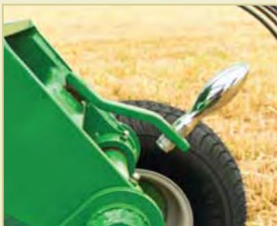
On the RR2109, use the rear height adjustment screw to distance the tines off the ground for less wear and tear. Also, you can set the height of the tines for optimal performance in a variety of crop conditions.
