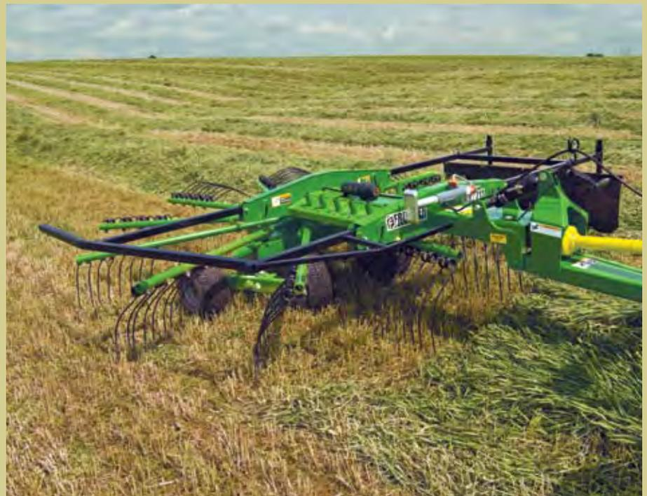
The RR2211 Rotary Rake has an 11-foot raking width for greater coverage. Hook this implement up to your small utility tractors with minimum 40 PTO HP. And for your convenience, the RR2211 tine arms can be removed and the guards folded up to obtain a narrow 5-foot transport width.
