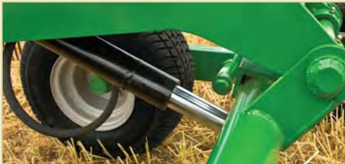
The hydraulic lift lets you raise or lower the rake for transport, and gives you greater maneuverability around the field to prevent windrow damage.
