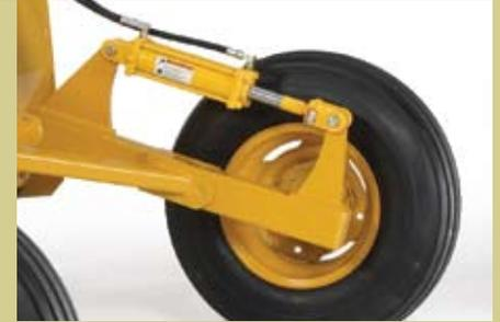
Tilt adjustment (*optional*) lets you angle the machine six inches to the left or right for a more aggressive cut when crowning roads or cutting ditches. Large flotation tires reduce scraper imbalance to maintain a smooth, stable ride for a quality cut on each pass.
