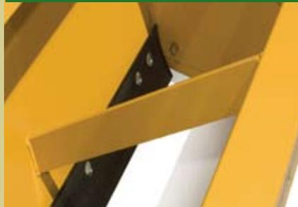
Internally braced steel plate moldboard is ¼-inch thick to add extra strength and rigidity for high hours of tough grading jobs.
