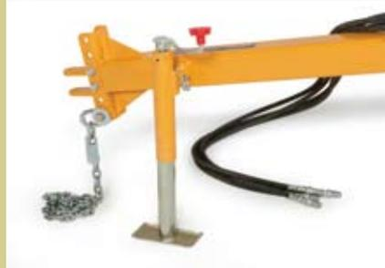
Adjustable clevis hitch keeps the scraper level with your tractor, preventing material loss and side plate wear. Safety chain comes standard.
