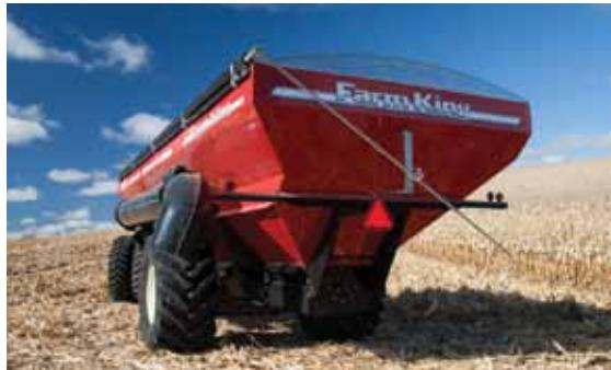
The Farm King grain cart builds on decades of high quality grain handling equipment manufacturing. Farm King products handle grain from the combine to market. Featuring a high capacity 21.5" unloading auger, standard roll tarp and a rotating unload spout. The Farm King grain cart also features a gravity flow discharge designed to unload directly into pits and auger hoppers. The 1060 and 1360 carts use high quality components and are built to handle the toughest harvest conditions.
