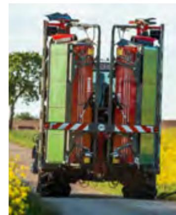
A computer-assisted automatic folding function with hydraulic transport lock allows for easy changing to the transport position, and protects the machine's power train from damage.
