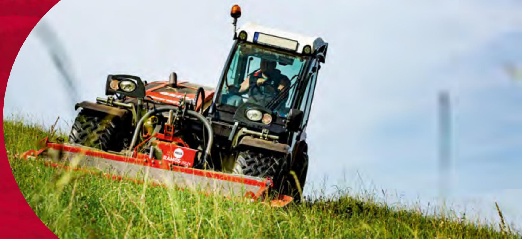
To also meet the high demands of farmers in alpine regions, FELLA has developed the RAMOS 200 series disc mowers. These are unique with their short, compact linkage. The centre of gravity lies close to the tractor and this leads to very good track stability on sloping terrain.
