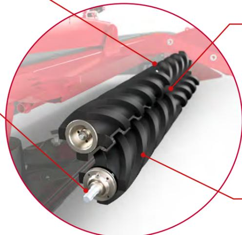
The contact pressure of the rubber profile elements can be variably adjusted to various forage and weather conditions.
