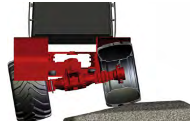
The rear axle is oscillating for best stability. The optional suspension gives safer and more comfortable operation.
