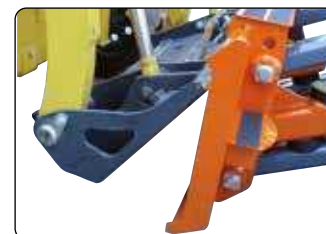
Linkage SAE J2513 with self levelling device.
