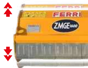
Floating frame following the ground contours
