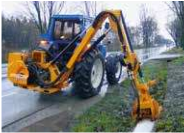
DITCH CLEANER FF45- FF60 For the maintenance of ditches Width 18" & 24"
