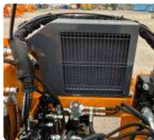
Oil cooler with thermostat.
