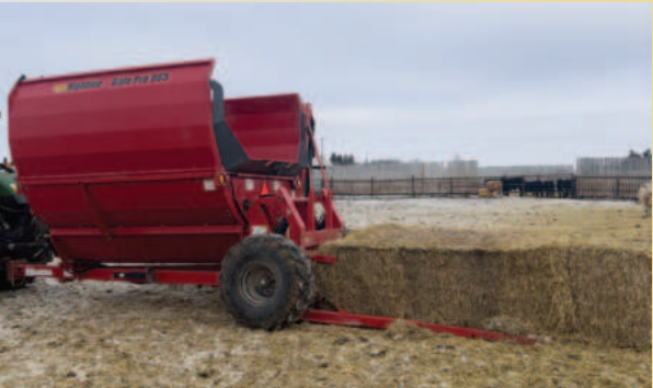
Lloads large square bales lengthwise.
