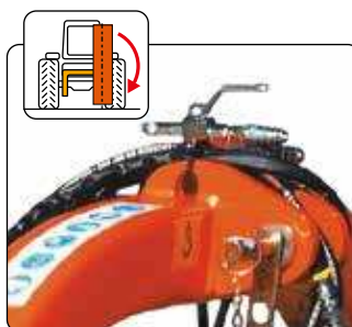
Hydraulic block tap for transport with manual activation (no chains or holders).
