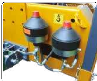
Lift float nitrogen accumulator.
