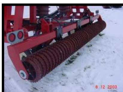
5 bearing main frame section, lights & reflectors standard
