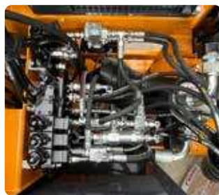
High Power Gear hydraulic system.
