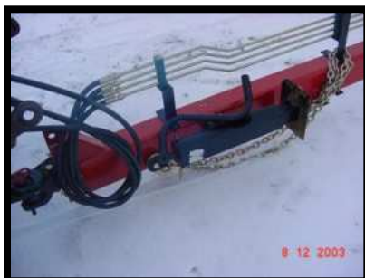
Adjustable clevis hitch, safety chains, 7000 lb tongue jack, steel hydraulic lines
