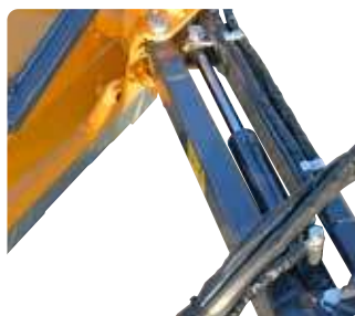
Hydraulic side shift cylinder fitted within the parallel arms for better protection during work.
