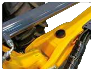
Drop forged arm brackets.
