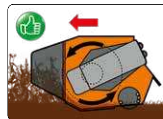
Rotor direction for grass and bushes.
