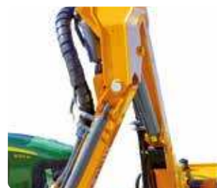
Hydraulic breakaway on second arm with accumulator controlled autoreset facility.
