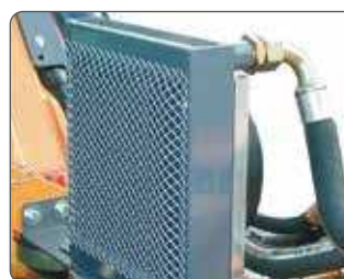
Oil cooler with thermostat (option).
