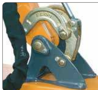
Drop forged lever for flail head rotation.
