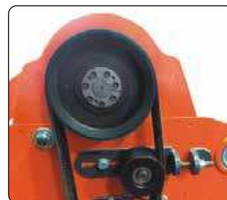
Belt drive with 4 or 5 belts and tightening pulley.
