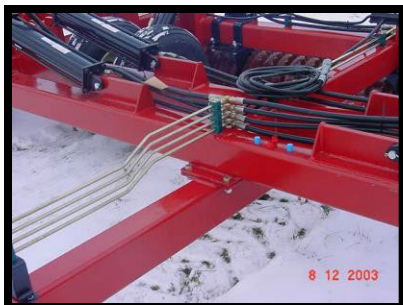
All plumbing neatly arranged and tied in place
