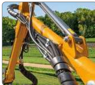
Arms with circular section H.T.R. (High Torsion Resistance).
