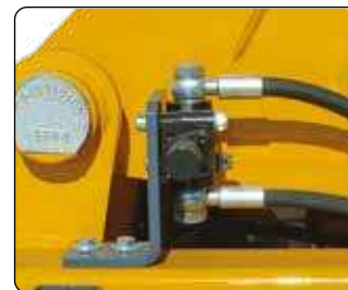
Single acting- double acting automatic switch.
