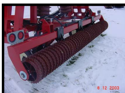
5 bearing main frame section, lights & reflectors standard
