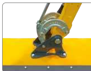
Drop forged flailhead linkages.
