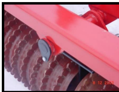
Rugged 1 3/4" hinge pins, securely fastened
