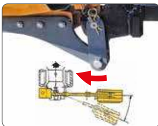
Mechanical breakaway (arm protection in case of obstacles).
