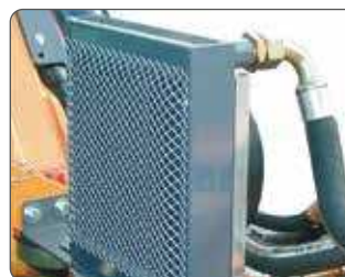
Oil cooler with thermostat (option).
