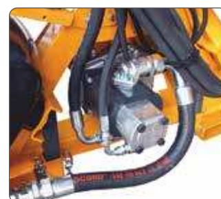
Group 3 cast iron hydraulic rotor pump.
