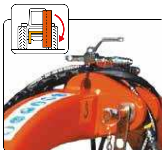
Hydraulic block tap for transport with manual activation (no chains or holders).
