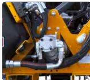
Aluminium rotor drive hydraulic pump.
