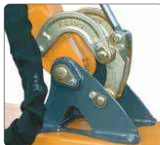
Drop forged lever for flail head rotation.
