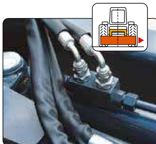
Hydraulic block valve for transport with automatic activation (no chains or holders).
