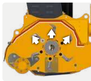
Inner lining "Full coverage" Domex 700 Steel.
