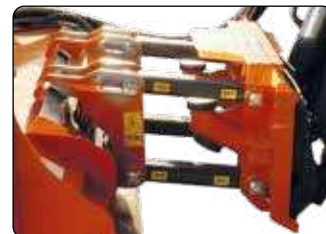
Parallel linkage for better floating on uneven grounds
