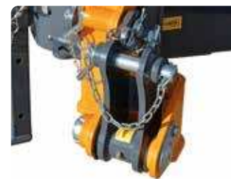
Mechanical shock absorber device (protection in case of obstacles).
