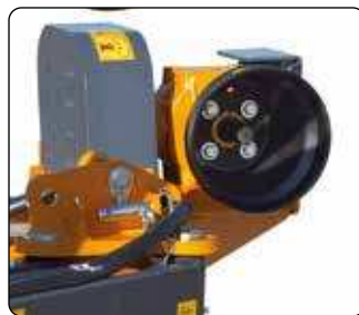
Gearbox external to the drive housing.
