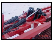
Rugged 4 beam main with section with two cylinders
