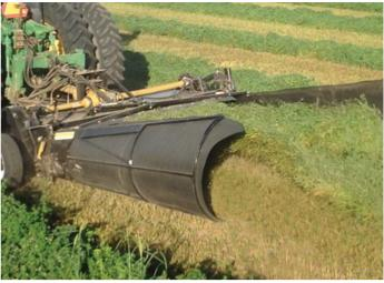
**Recon 400** - 3 point hitch has a pivoting body that allows you to angle the machine 25 degrees to combine two swaths to save a raking pass.
