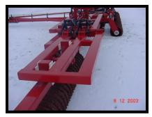
3 beam outerwing section w/ two cylinders, each packer gang oscillates on centre pin and plastic wear plates
