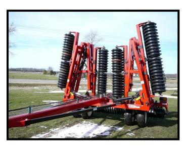
Flex packers are available in a 3-section configuration for widths of 21' to 32' (shown on left). Packers 33' to 50' are built on a 5-section frame (shown right). The balanced frame design minimizes tongue weight.
