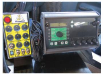
Optional Microtrak autorate controller provides accurate product application. All functions are remotely controlled from the cab by electric solenoids.
