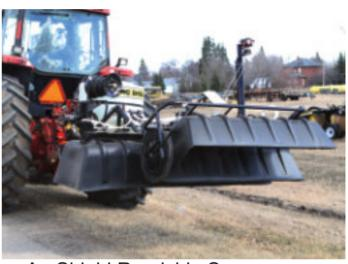
Ag Shield Roadside Sprayers are designed for easy transport. Simply fold the boom(s), lock into place and drive to the next job site.
