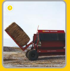
The bale is aligned with the flail drum for efficient processing.
