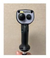
Easily and accurately position the discharge chute from the tractor cab for accurate placement of feed or bedding. With a wide range of motion (chute rotates 130 degrees left and 130 degrees right, as well as 25 degrees up and down), the discharge chute (84" (2.13 m) long, 11' (3.35 m) high nozzle) can be directed to throw material up to 80' (24.3 m)\*. NOTE: Right/Left hand is determined by sitting in the tractor seat looking forward.
