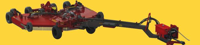
An industry exclusive feature of a Highline<sup>®</sup> mower is the integrated Radial Contouring Hitch (RCH<sup>™</sup>). The RCH<sup>™</sup> is designed to keep the tractor on the road and the Operator safe while achieving a quality cut.
