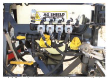
All functions are remotely controlled from the cab by electric solenoids. Premium hand wand & reel (optional).
