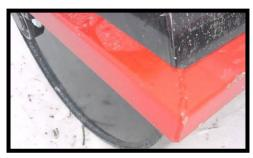
The **Extra Heavy-Duty** frame is made of 2" square tubing that is 3/16" thick. It has mitered corners and surrounds the drum for added strength.
