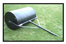
The drum is made from tubular steel 30" in diameter and 3/8" thick. The end plates are 10-gauge steel with 1" bearing on the standard roller. The Extra Heavy-Duty version uses  $\frac{1}{4}$ " steel with 1  $\frac{3}{4}$ " pillow block bearings.
