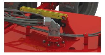
The hydraulic drive advantage translates into less time doing maintenance and more time operating! This is because the hydraulic drive system eliminates a number of moving parts including slip clutches which can wear over time reducing overall performance. Also, when a mower blade hits an obstacle, the hydraulic pressure is relieved, reducing force being applied on the blade and potential damage.
