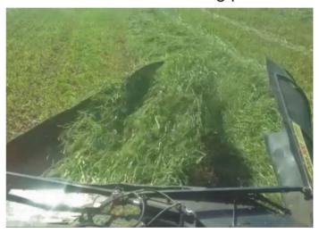
Side deflectors invert and move the swath onto dry ground to speed up the drying process and at the same time adjusting swath width to match baler.
