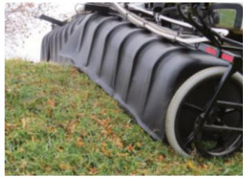
Ag Shield Roadside Sprayers feature a breakaway boom with gauge wheels at the center and outer edge to ensure the boom follows varying terrain. This design ensures that sprayer shield stays in close proximity to the ground, maximizing drift control and safety.
