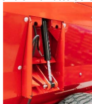
Hydraulic Bale Lift Plates SC4902
