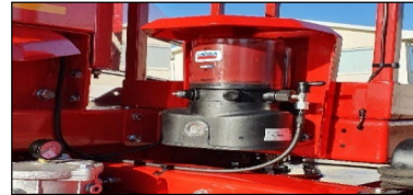
NEW : Auto Greasing System as Standard
