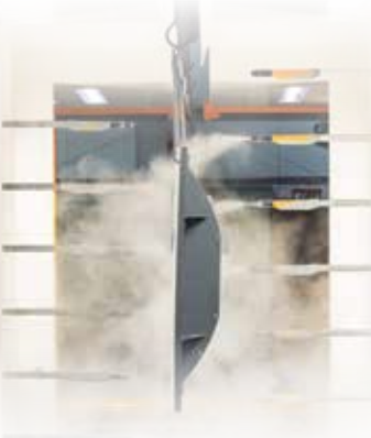
State of the art automated Primer Powder Booth
