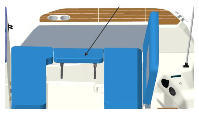
• Counter drill the bracket as far to the rear as possible with a  $\emptyset$ 4.5 mm drill bit
