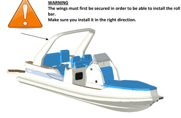
Apply SIKA on the feet of the roll bar. Leave 10 to 15 mm clearance around the edges of the feet so the SIKA doesn't squeeze out when you tighten it down.
