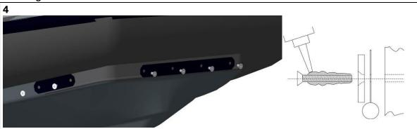
Place the buoyancy tube and make fast the outer flap (buoyancy tube deflated) using the stainless steel bars and the screws supplied in the buoyancy tube kit. To ensure that the assembly is mechanically secure, apply medium strength threadlocker to the screws.
