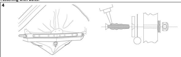
After inflating the buoyancy tube (see the chapters below), secure the outer flap using the stainless steel bars and screws provided in the buoyancy tube kit. Apply sealing compound on all the screws and in the hull holes to achieve watertightness.
