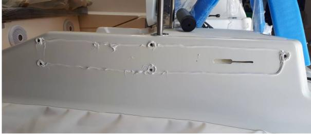
• Place the wings on the deck and secure them with screws, starting from the front.
