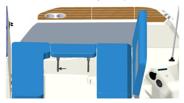
Inject SIKA sealant into the hole to ensure watertightness and secure with a sheetmetal screw.
