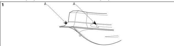
In order to facilitate the fitting of the buoyancy tube, apply liquid soap to the hull's rails (A).
