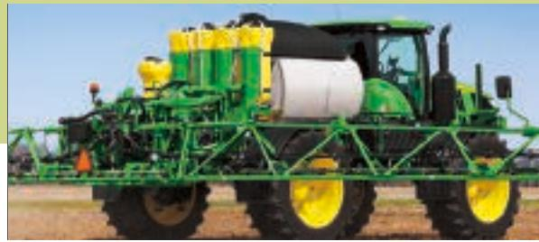
**Direct Injection system** (available on R4030, R4038 and R4045 Sprayers) increases your flexibility by changing rates and products on the fly without stopping to mix products. The integrated system injects products directly into the system at the boom. The results: quicker changeovers, increased flexibility and lowered risk of using multiple products.
