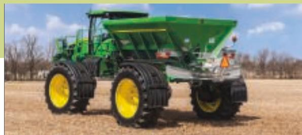
\*5 ft. dual bin insert with 66 cu. ft. (1.87 cu. m) capacity on DN456 and 106 cu. ft. (3.00 cu. m) on the DN485.
