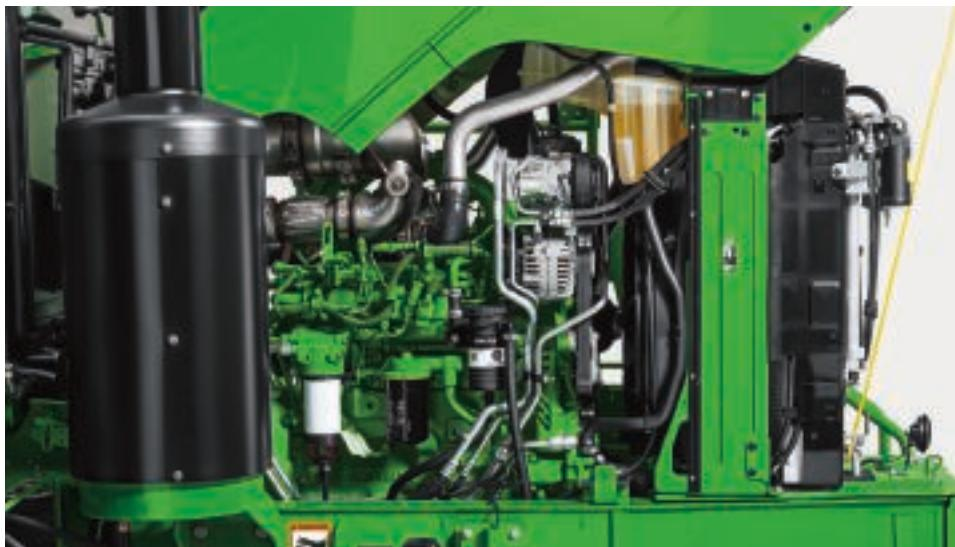
**Final Tier 4 engine** is rated at 173 hp (129 kW) and boosts power 5 percent more than our former model. This 4.5L engine is designed to increase power bulge from 173 to 182 hp (136 kW) with a 10% gain in peak torque. That's dependable power in harsh conditions to let you spray at higher speeds than before.
