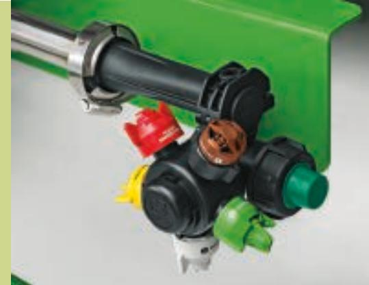
**End cap aspirators** on the end of each spray section reduce nozzle turn-off time by up to 85% and terminate dead ends that can collect unwanted product residue. Available in both standard- and high-flow plumbing options – or stainless steel or poly options – this feature rids dead end space and allows air to be expelled.
