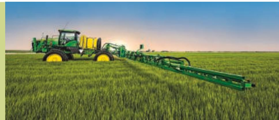
**Proven design.** We realize carbon fiber isn't ideal for all situations, and that's why we rely on the proven design of our steel booms to get the job done. The rock solid construction includes a reliable dual swing link suspension and greater stability while delivering consistent height above crop, acre after acre. And the flat-fold design lets you spray up to 120 ft. (36 m) wide.
