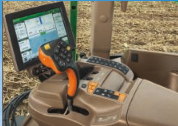
A high-resolution 10-inch GreenStar™ 4600 CommandCenter™ display and the smartly configured CommandARM™ for fingertip control of important functions.
