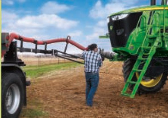
**Exclusive Load Command™ system** dramatically cuts loading time on the R4045 Sprayer only. Load the 1,200-gallon (4,500L) tank as fast as three minutes. System automatically disengages when your sprayer tank is full. Plus, there's reduced risk of any product exposure.
