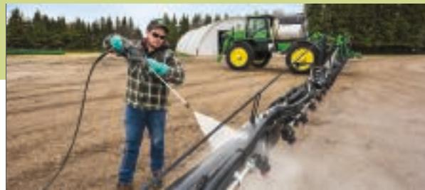
**Built to last.** With a higher strength-to-weight ratio than steel and aluminum, carbon fiber is also corrosion-resistant and easy to clean and maintain.
