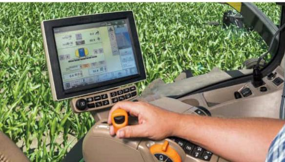
*The 2530L comes standard with a GreenStar Rate Controller for full one-step integration of the GreenStar Display with the liquid system. This integration enables features like automatic rate control, field documentation, map-based prescriptions and John Deere Section Control (activation required).*
