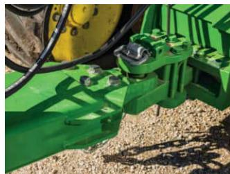
**The floating hitch and flexible frame** maintain consistent ground contact and uniform depth. The four-rank frame allows for high levels of residue to flow smoothly through staggered row-units, reducing downtime from plugging.
