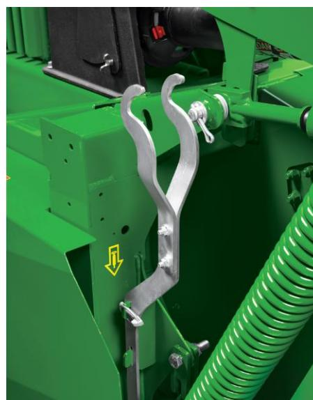
Change knives in minutes, using only this quick change tool, which attaches to the back of the Mower-Conditioner for easy access.
