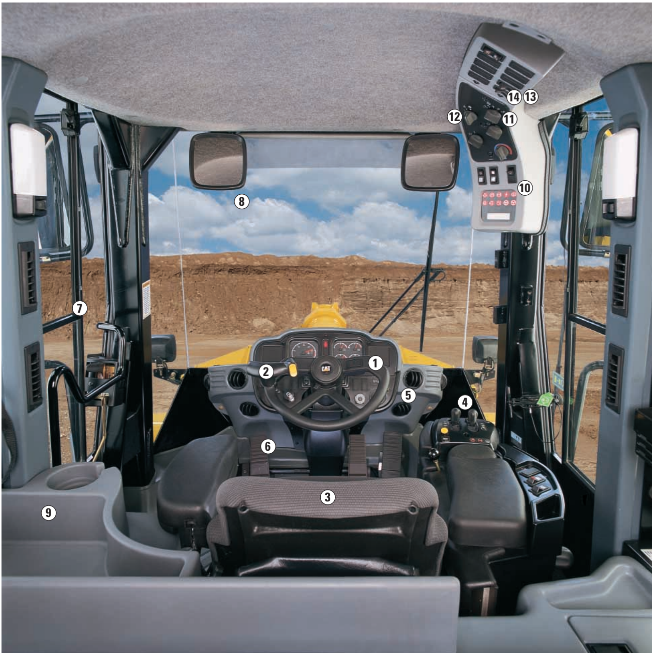
Command Control Steering with Electro-Hydraulic Bucket Controls
