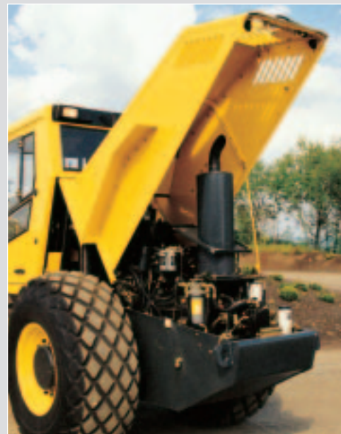
Large steel engine hood provides easy access to all service and maintenance points
