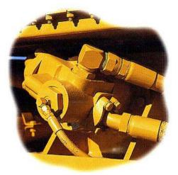
The main hydraulic/steering pump is a load-sensing gear-type pump chosen for extended service life and low replacement cost. Gear type pumps are more tolerant of fluid contamination, perform better in cold weather, and are easier to service than piston pump designs.
