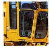
Series IV cab changes include a 'sweep-out' cab floor, easy-to-use door releases and re-enforced door and window frames. Twopiece door glass design makes glass replacement easier and less costly than ever before!
