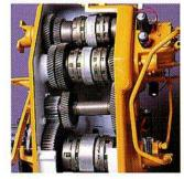
The exclusive **Champion 8400** grader transmission is now in service in more than 10,000 units. Evenly proportioned gear ratios provide precise, job-matched speeds for any grading application. A new "Smart Shift" feature lets the operator easily customize shift patterns to the job at hand.
