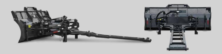
Pitbull's unique Undermount system for All-Wheel Steering tractors offers a new breed of dozer blade performance. When removing the blade, the lift assembly tucks tightly against the nose of your tractor for clear sightlines and easy road travel. The full undermount disconnect is also a simple process, with only a few coupling brackets remaining as your tractor is restored to near original ground clearance.
