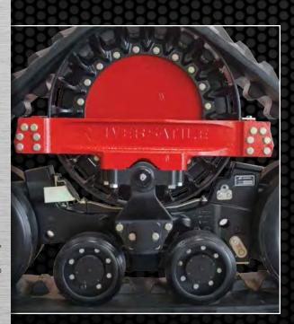
the tractor. The frame absorbs stress from each track to increase track system life and reduce maintenance requirements.
