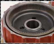
The DeltaTrack was designed using the legendary Versatile outboard planetary system. In addition to doing a better job of putting power to the ground the outboard planetary is far easier to service than competitive inboard units. Removing the planetary cover exposes the planetary gears and sun gear for easy access.
