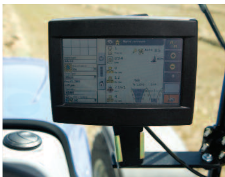
You monitor and control bale density from your seat (IntelliView™ III monitor shown).
