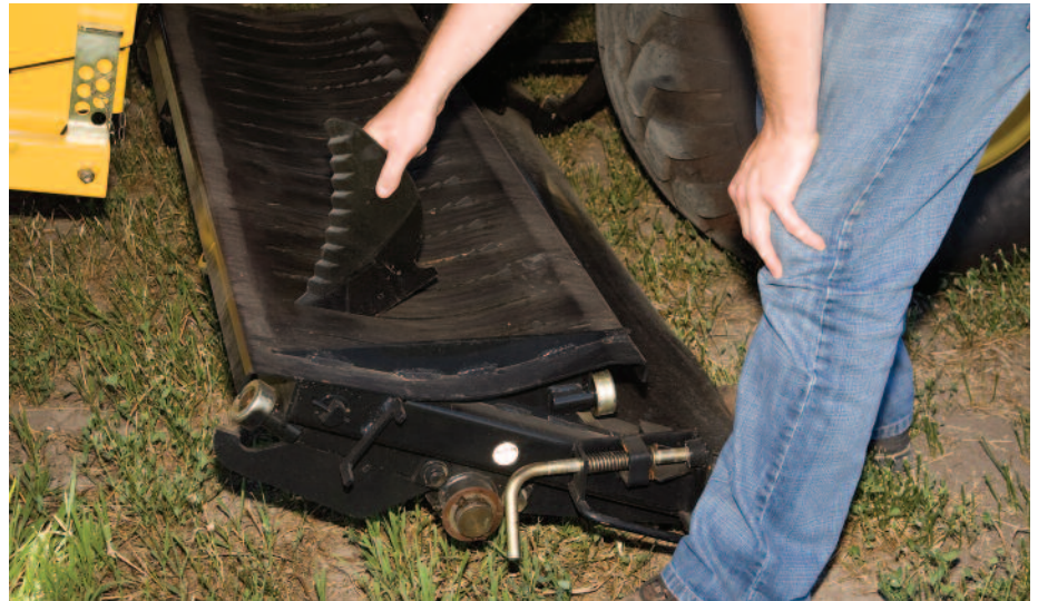
Knife sharpening is easy, so your operators are more likely to do it when needed, resulting in smoother cutting that requires less power. The Rotor Cutter knife drawer slides out for fast knife inspection and sharpening.
