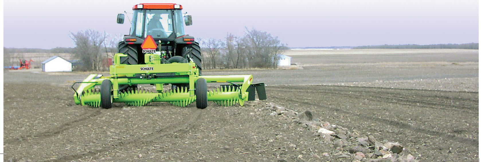
SRW-1400-H Features a hydraulic chain drive system
