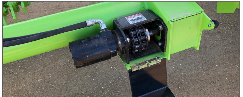
SRW-1400-H Features a hydraulic chain drive system
