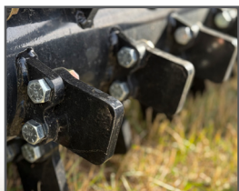
4" Replaceable teeth 450 BHN steel
