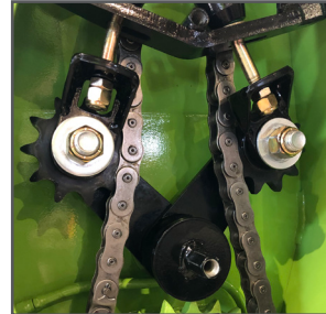
Chain case with tensioner and heavy #80 chain which is run in an oil bath and accessible with an easy access cover plate.
