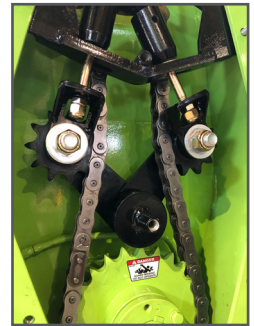
Chain case with tensioner and heavy #80 chain with easy access opening plate.
