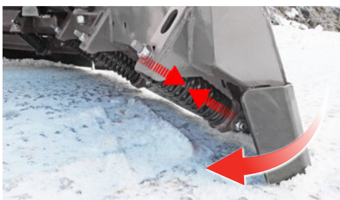
Cutting edge with trip springs
