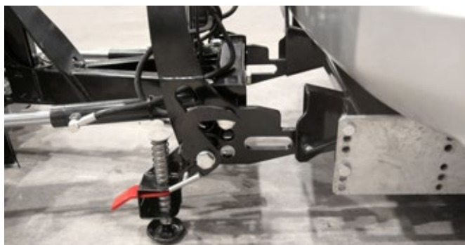
Quick hitch - lift shoe handle to attach your plow to the vehicle
