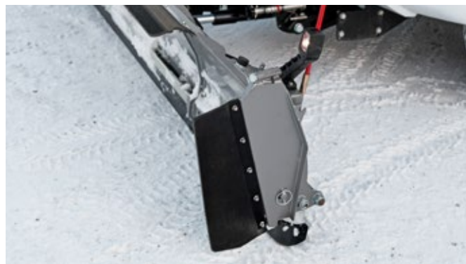
End guiding plate and LED edge-marker
