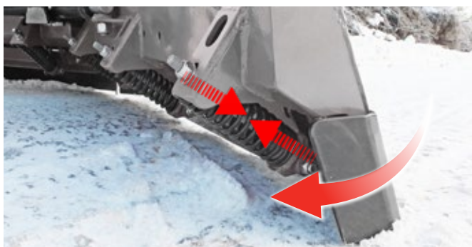
Cutting edge with trip springs
