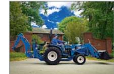
Optional quick attach backhoe Remove or attach in seconds. With 76" digging depth, 2,817 lbs of digging force and 180° swing arc, it outperforms other in its class
