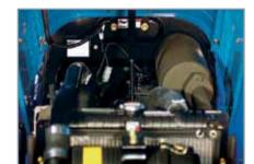
LS Tier 4 Interim Engine 3 cyl, low vibration, fuel efficient yet powerful
