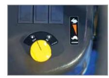
PTO On/Off Switch Turn the independent rear PTO on or off with a simple push of a button
