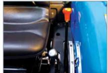
Simple gear range selections Select your gear range or 2WD/4WD with simple move of the levers
