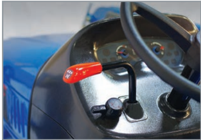
Synchro Shuttle lever Makes changing direction easier than competitive non-shuttle gear models
