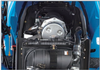
Eco-friendly ISM Tier4 Engine NEW, powerful and clean electronic engine with DPF
