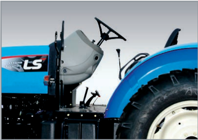
Spacious Flat platform With side mounted gear lever, maximizes space and makes getting on/off tractor easier
