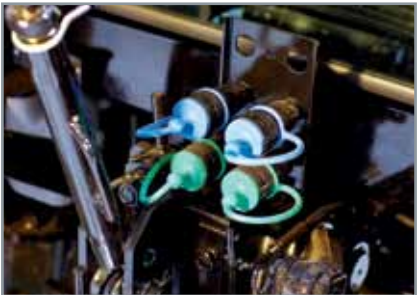
2 sets of remotes and detent function standard Adds functionality and improves ease of use by allowing attachment of hydraulically controlled implements without the high, additional costs like others in its class to add the remotes as options
