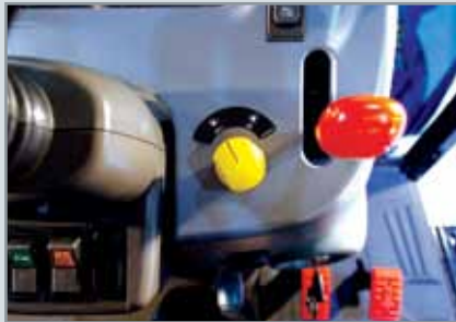
PTO Switches Select manual or independent PTO (non HST models only) and turn on or off with a simple turn of switches
