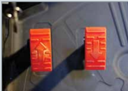
Hydrostatic Transmission Models Maximizes ease of use with effortless, clutchless and instant speed and directional changes with a simple push of the pedals
