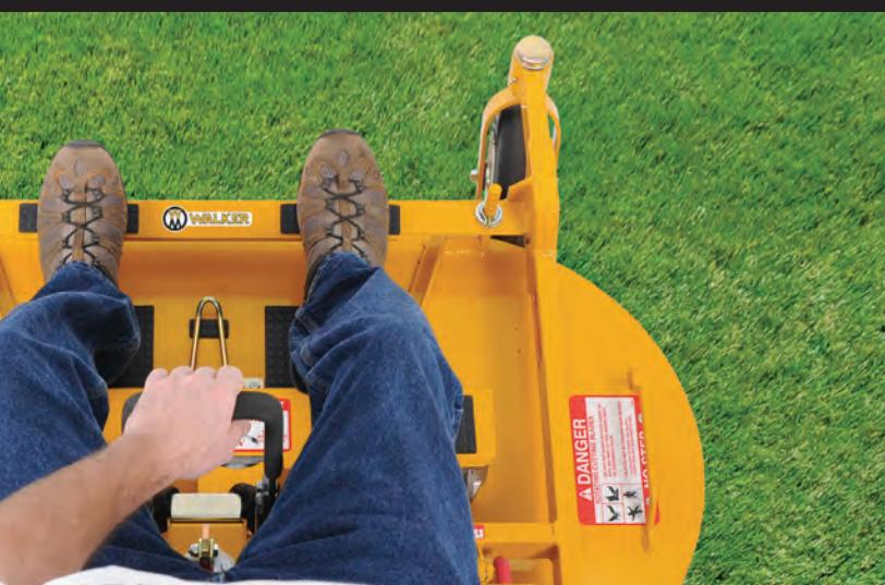
While other mowers use lap bars and arm movements to steer, the Walker uses a forward speed control/cruise control and gentle fingertip pressure on the steering levers to precisely maneuver the machine.
