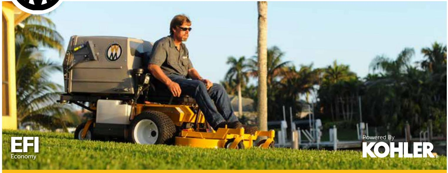
**Operators can expect easy starting, consistent running temperatures, and user-friendly maintenance from this top-of-the-line mower. A combination of liquid cooling and EFI from Kohler's 30-HP Aegis engine provides increased engine life, power, and better fuel economy compared to air-cooled engines.**
