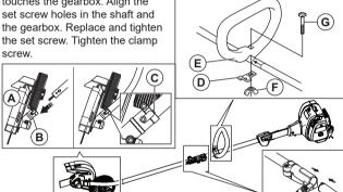
Push the shaft into the coupling until it clicks in position.
