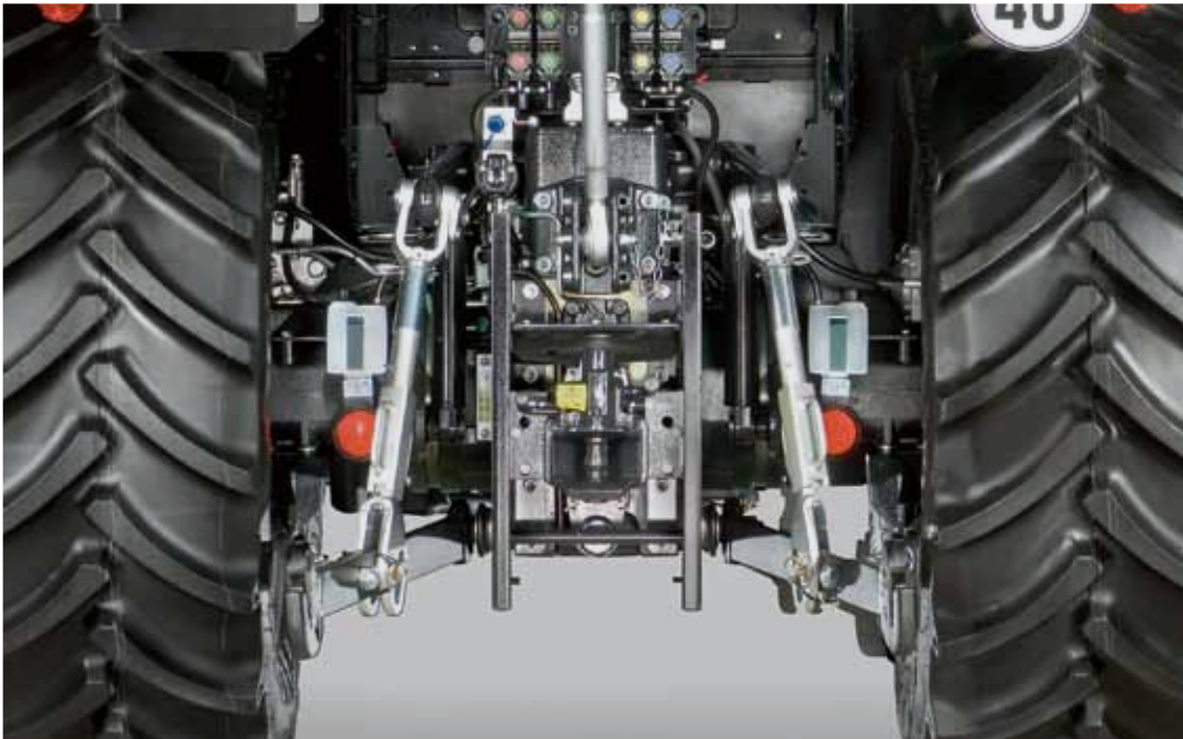
The powerful rear linkage with 6,200 kg lift capacity for operating the heaviest implements.
