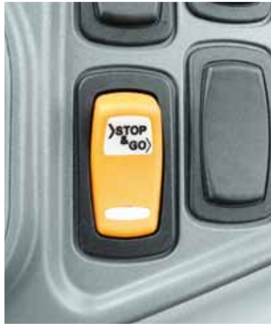
Stop & Go is activated per toggle switch.
