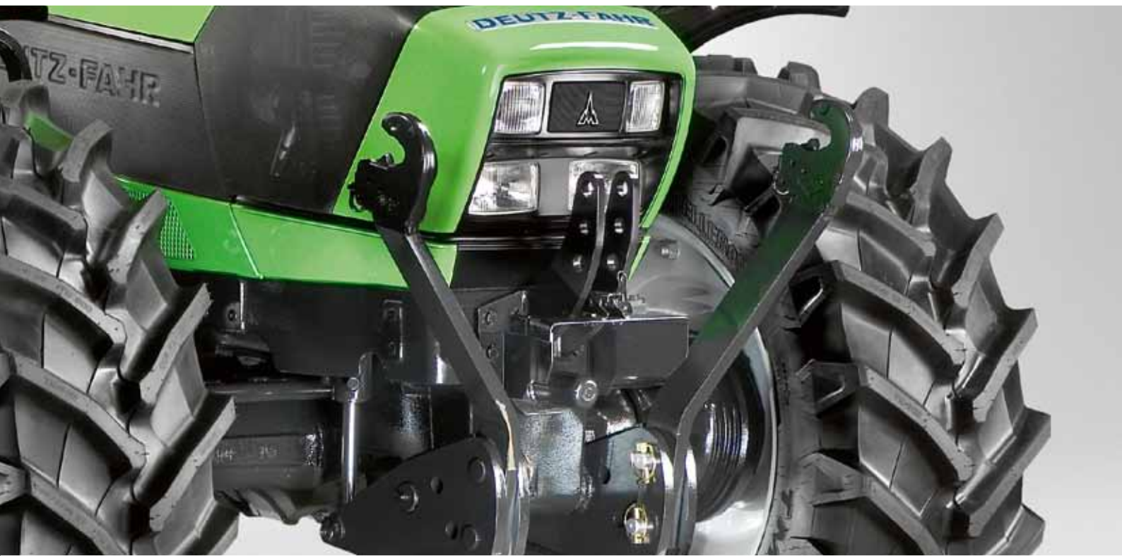
Fully integrated, powerful front hydraulics with 1.8 t lifting force.
