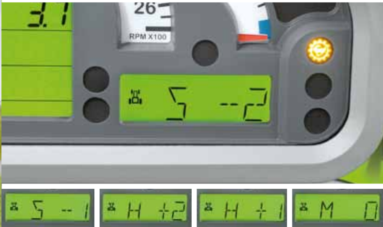
Modulation of powershuttle is shown on the display.
