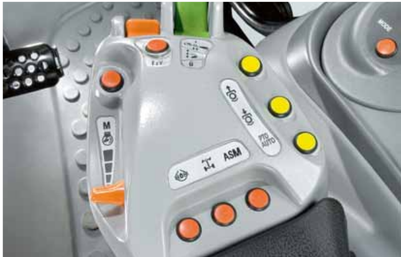
Electro-hydraulically operated PTO (push-button control).
