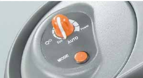
Stepless adjustment of engine and transmission management.
