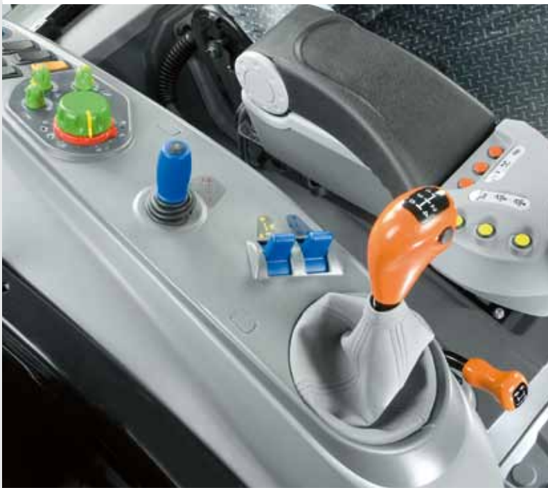
Operation of the comfort clutch using a button in the switching knob.
