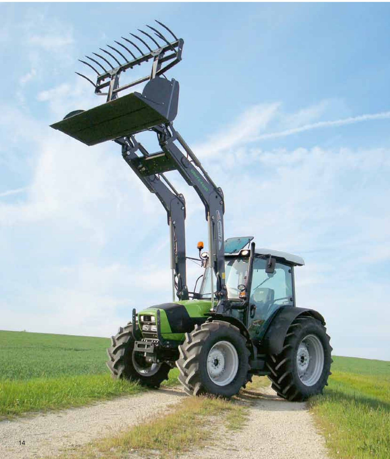
Fully integrated, powerful front hydraulics with 1.8 t lifting force.
