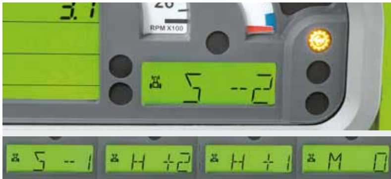
Modulation of powershuttle is shown on the display.
