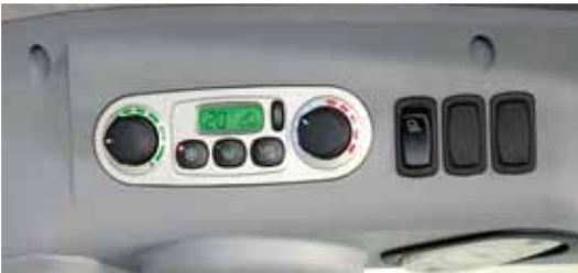
The controls for the heating and air conditioning system are installed in the roof. The air conditioning system is a standard feature. An optional electronically controlled automatic air conditioner is standard for the "ProfilLine" version.
