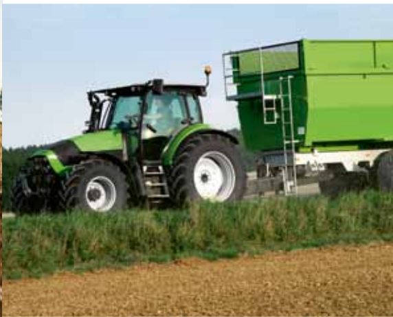
Road transport. The advantages of ASM: Speed above 15 km/h – 4wheel drive disengaged; Speed below 14 km/h – 4wheel drive engaged.
