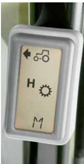
Everything in sight: The central display in the A-post shows the activated Powershift stage.
