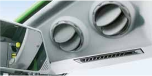
A total of 17 air nozzles ensure excellent cab ventilation and quick demisting.
