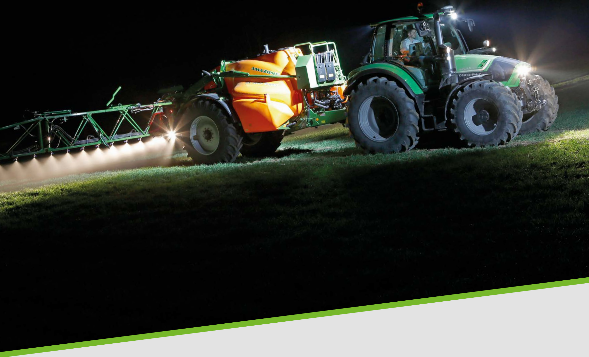
Automatic control of the partial sections when entering or leaving the field or working on wedge-shaped sections.
