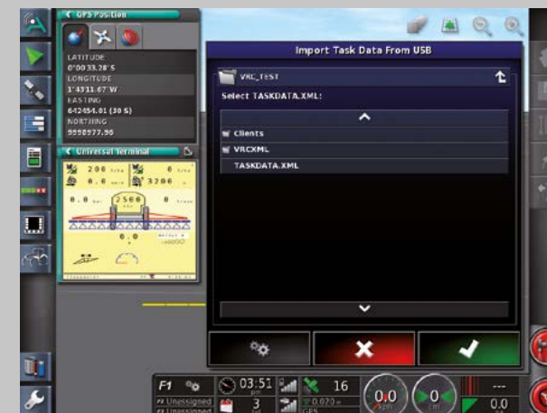
Data management: the ISOXML standard allows for compatibility with FMIS.
