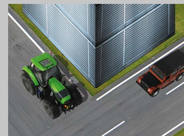
At dangerous junctions, the system extends the driver's angle of view and displays traffic that the driver could not see without pulling out further.
