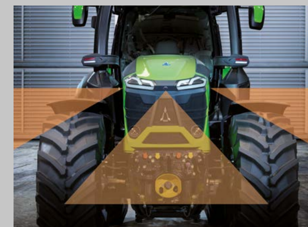
Active detection and warning when a person is in front of the tractor.
