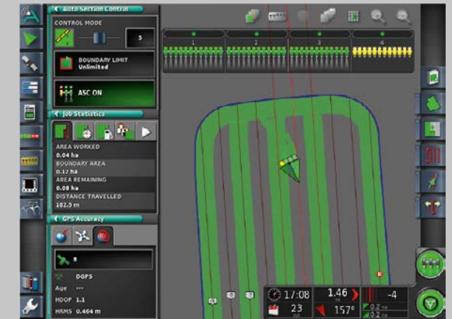
Partial sections are switched automatically but can also be switched manually via the virtual display.
