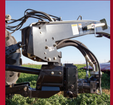
MacDon's APT hitch allows you to pull the machine on either side of the tractor for back and forth harvesting.
