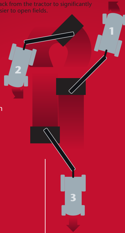
MacDon's APT hitch allows you to pull the machine on either side of the tractor for back and forth harvesting.
