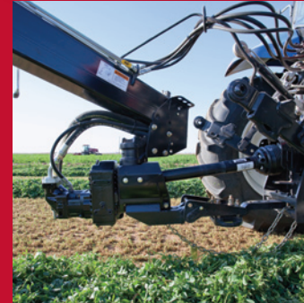
MacDon's APT hitch allows you to pull the machine on either side of the tractor for back and forth harvesting.
