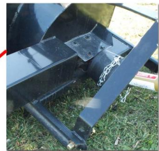
Heavy duty PTO with needle bearings
