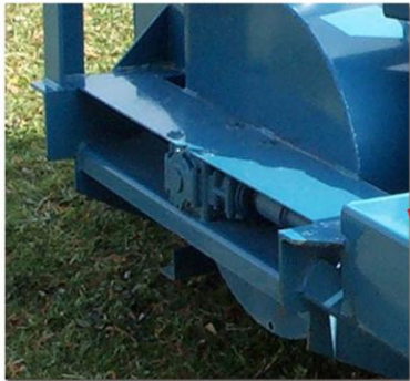
Heavy-duty gearbox with heat treated gears and tapered roller bearings
