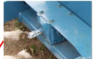
Heavy-duty gearbox with heat treated gears and tapered roller bearings
