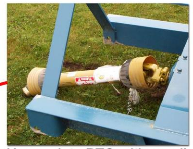
Heavy-duty PTO with needle bearings
