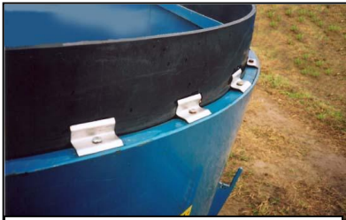
9" rubber extension for larger capacity mixes
