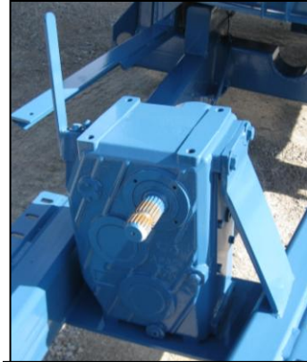
2-speed gearbox for better mixing power (optional on 2260 & 2270)
