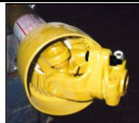
PTO drive assembly with shear bolt for equipment protection
