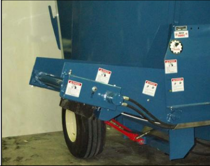
Hydraulic raise and lower discharge conveyor extensions
