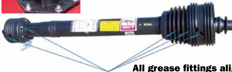
Bush Hog's E-Z lube drivelines are quick and easy to service. All grease fittings on the PTO CV driveline and wing drivelines align for quick location of grease points. Since all grease fittings on all drivelines are in an up position on every 5th revolution, service times are reduced.
