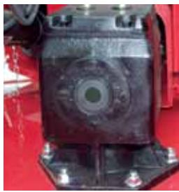
The Patent Pending oil sight gauge takes the guess work out of checking the oil. In less than 10 seconds, all three cutting box oil levels can be checked and rechecked as often as you walk around the machine. Never climb onto the cutter again to check the gearbox oil levels.
