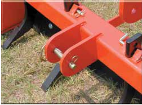
Scarifiers can rip soil up to 2-3/8-inch deep
