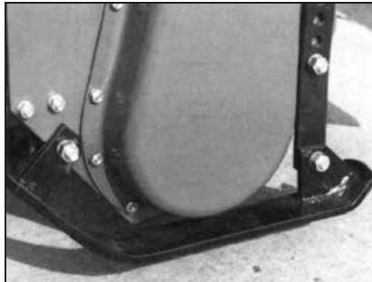
Adjustable skid shoes are standard equipment for precise depth control. RTH, RTN, and RTNR tillers adjust through 5 positions to a 7-inch tilling depth and RTS tillers adjust through 4 positions to a 7-inch depth.
