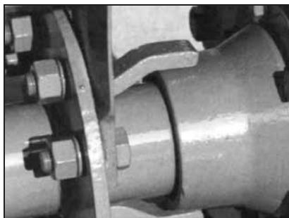
A unique anti-wrap device on the RTH and RTN tillers prevents residue from damaging seals. On the RTS tillers, triple-lip sealed ball bearings on the rotor shaft help keep dirt out and reduce wrapping.
