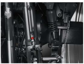
SPRING-MOUNTED CAB & SPRING-MOUNTED FRONT DRIVEN AXLE
