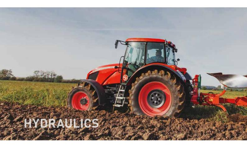
Forterra tractors are equipped with EHR (Bosch electrohydraulics) with Hitchtronic function. Two auxiliary hydraulic cylinders ensure uniform tractor loading and maximum lifting capacity up to 77 kN for Forterra CL and up to 85 kN for Forterra HSX and Forterra HD. Forterra HD offers four auxiliary hydraulic quick couplers with electro-hydraulic control. In combination with Category III hitches, you can enjoy a wide selection of usable implements.
