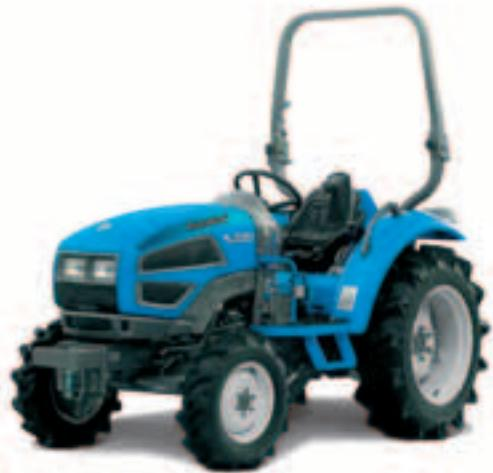
Specially designed to perform light farm tasks as well as lawn and maintenance jobs, the 1-30 and 1-35 tractors provide outstanding agility and easy manoeuvrability. Both series are powered by 3-cylinder water-cooled engines that deliver 28 and 34 hp respectively and meet the Tier 3 emission standards.
