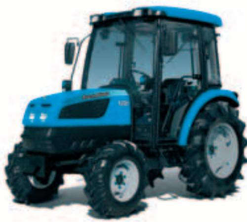
The 1-40 and 1-50 series tractors are designed to combine high performance, versatility and comfort in a compact footprint. They are powered by 41- and 49-hp, 4-cylinder, naturally aspirated diesel engines meeting the Tier 3 emission standards.
