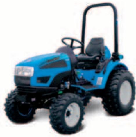
The small Landini 1-25 is specially designed to perform light farm tasks as well as lawn and landscape maintenance jobs. It is powered by a 3-cylinder, water-cooled diesel engine which delivers 22 hp and meets the Tier 3 emissions standards.
