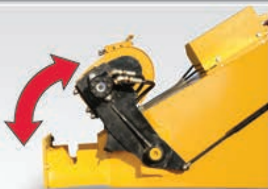
Lift assist for servicing using gas shocks.
